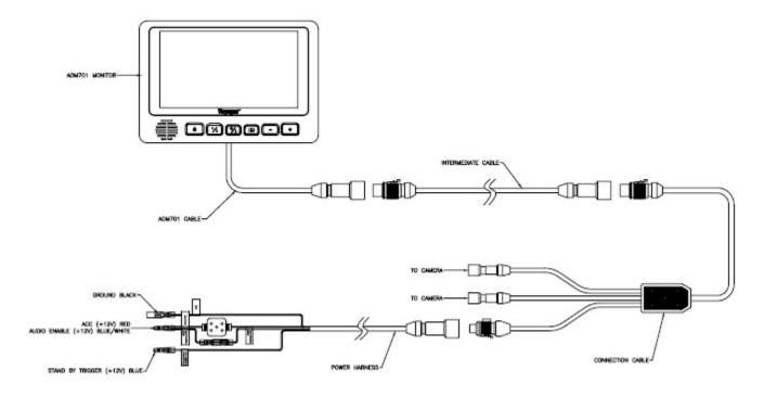
Install the **AOM713WP** monitor panel and junction box to the intermediate harness and power harness from the existing system. Your camera cable with connect into the **CA1**, **CA2**, or **CA3** inputs.
