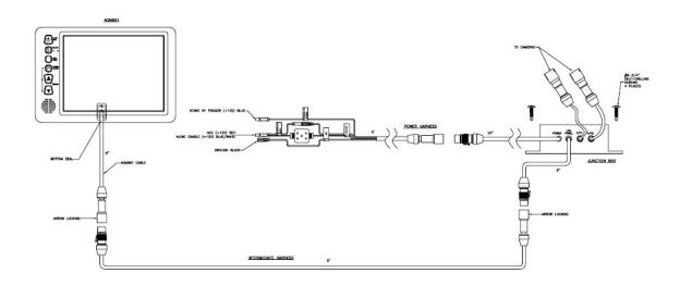
Install the **AOM713** monitor panel and wiring harness in place of the old system. Your camera cable will connect into the **TO CAMERA** inputs.
